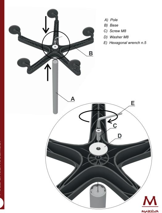
Insert the pole (A) in the special slots on the back of the body (F) and lock it with the screw (C) supplied, taking care to tighten the screw with moderation. Pay attention to the positioning of the base (see page's bottom)
